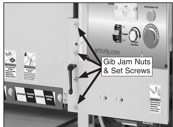
Figure 34. Gib jam nuts and set screws.
